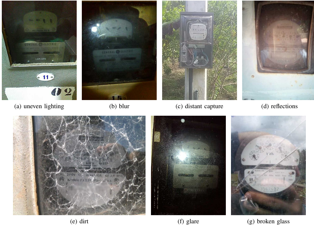
Fig. 4. Samples of the challenging scenarios present on the provided images. We selected for the UFPR-ADMR dataset 2,000 images in which it was possible for a human to recognize the correct reading of the meter. We blurred the region containing the consumer unit number in each image due to privacy constraints.
