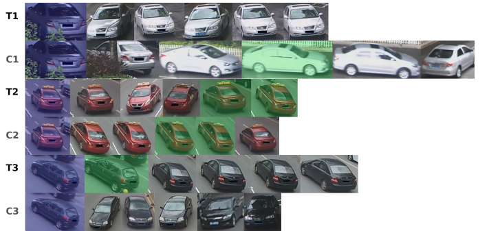
Fig. 3. Challenging situations found in both CL-NGT and TL-NGT. The query image is highlighted in blue, while the correct results are highlighted in green. The first two cases are difficult even for human operators: a careful examination is needed to understand why similar cars actually have different IDs. One can observe how hard is to find out that a little detail in the left rear window can evidence similarity between the correct results and the query image (T2 and C2). The image aspect ratio is kept for better visualization of differences. Best viewed in color.
