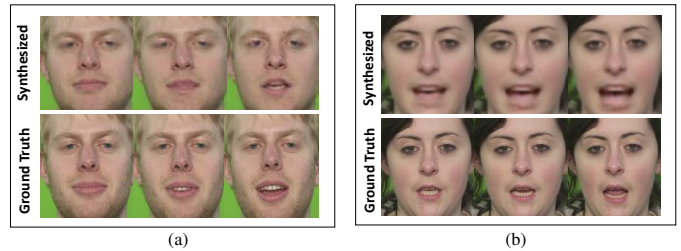
Fig. 1: Issues with current methods in 2D facial animation (a) Difference in image texture of synthesized face produced by Vougioukas et al. [27] from the ground truth image texture leads to perceived difference in identity of the rendered face from the target individual. (b) Despite synchronization with audio, the facial animation sequence synthesized using the method of Chen et al. [4] contains implausible or unnatural mouth shape (last frame) that can be perceived as being fake. The results were obtained by evaluation using pre-trained models made publicly available by the respective authors.
