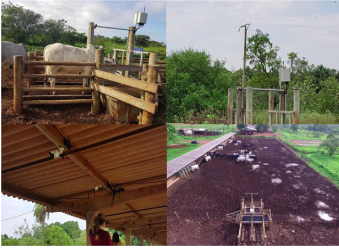
Fig. 2. Embrapa Beef Cattle image acquisition system - (a, top left) Intergado water trough, (b, top right) cameras installed on the water trough, (c, bottom left) cameras installed on the feeding troughs to capture profile images, (d, bottom right) aerial view of Embrapa Beef Cattle feedlot with the collection system.
