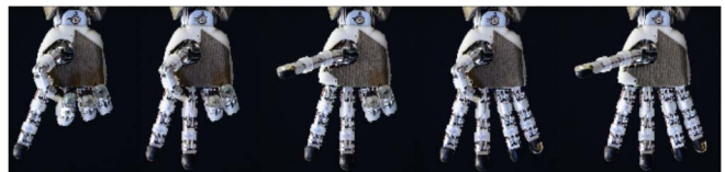
Fig. 1. The number representations with the iCub right-hand fingers. From one, two, three, four and five. Numbers from six to nine are represented with two hands, with the right hand fully open. In practice, the embodied inputs are the joint angles from the fingers' motor encoders.
