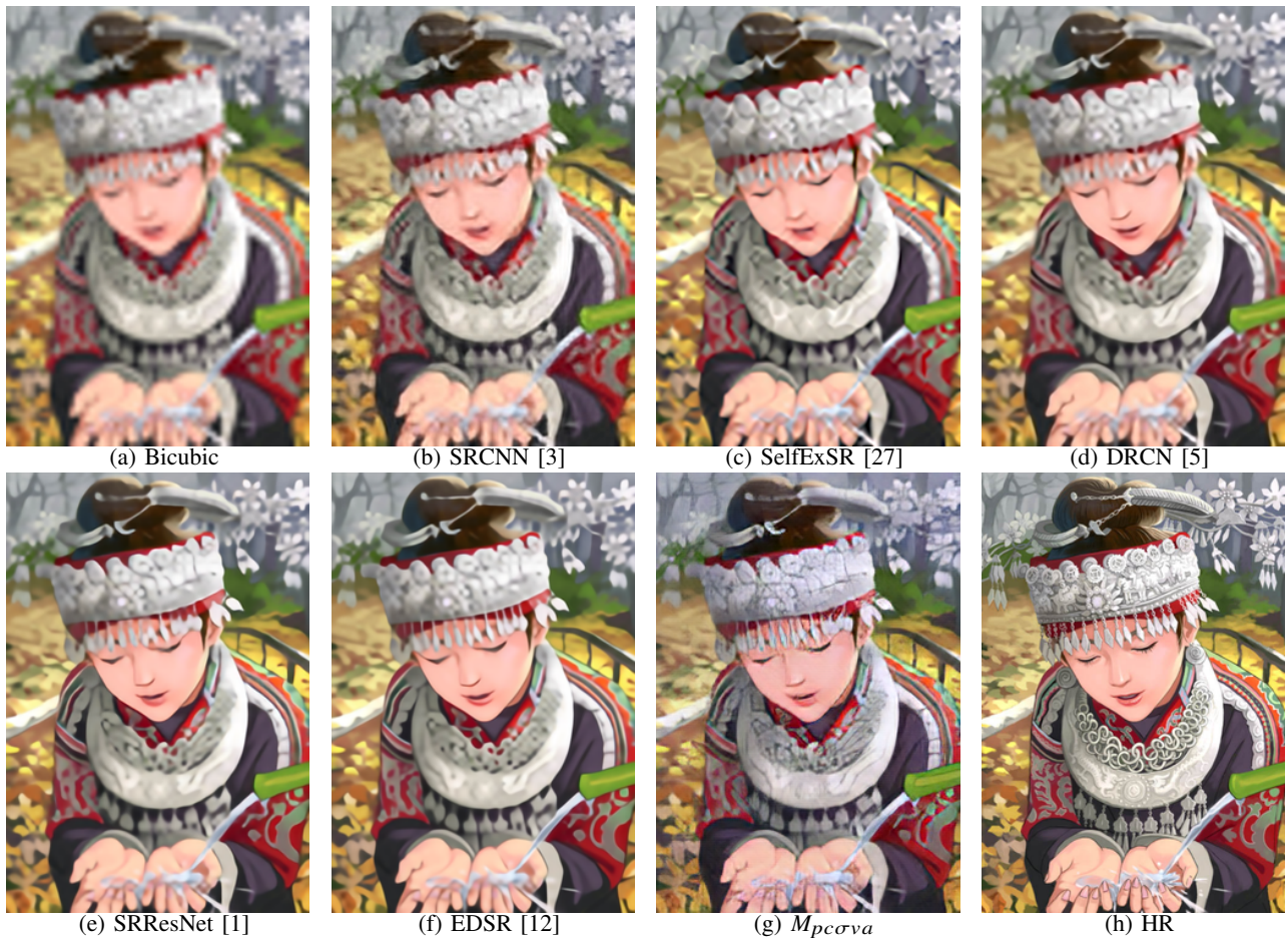
Fig. 5: Qualitative comparison of our method ( M_{pc\sigma va} ) with other SR models on the Comic image from Set14.
