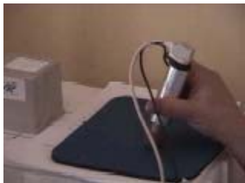
Figure 4: The pseudo haptic input device used to control the orientations and positions of the remote robot.
