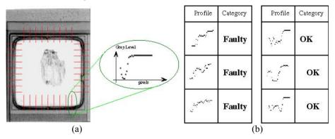
**Fig. 3.** Example of profiles extraction after via centring process (a). Example of profiles to category association during the learning phase (b).
