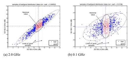
**Fig. 2.**  $S_{21}$  parameter relationships for the 2.4 GHz LNA model used in circuit simulations: (a)  $S_{21}$  @ 2.0 GHz and (b)  $S_{21}$  @ 0.1 GHz plotted against  $S_{21}$  at the operating frequency.
