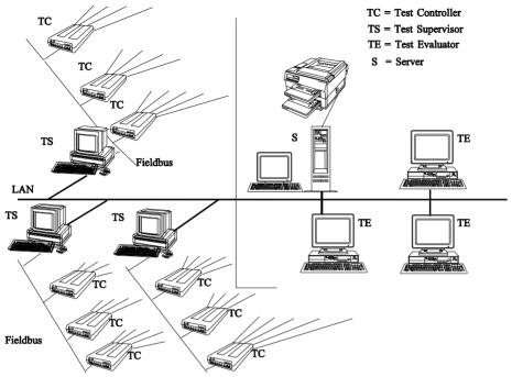
Fig. 1. Measurement system architecture.
