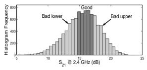
Fig. 3. Histogram of 'good' and 'bad' circuits as defined by the S<sub>21</sub> performance criteria.
