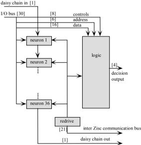
Fig. 2. IBM ZISC-036 chip's bloc diagram.
