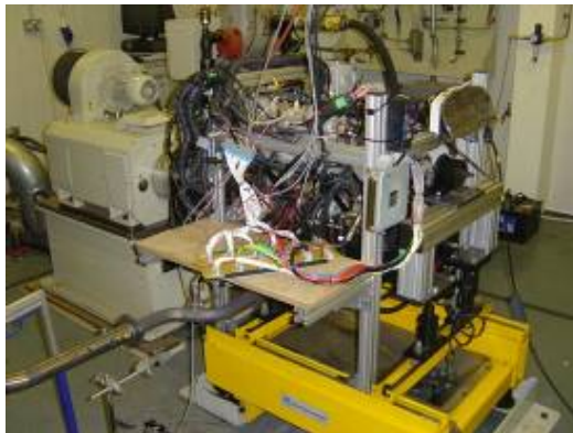
Fig. 1. View of engine test-bed and dynamometer.
