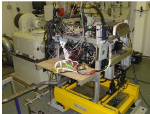
Fig. 1. View of engine test-bed and dynamometer.
