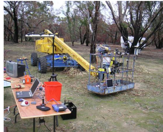
Figure 6(a): Teleoperated Boom Truck.
