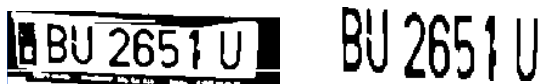
Figure 5: License plate before and after eliminating the black areas that does not correspond with characters.
