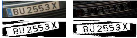
Figure 4: Top left: Original RGB image. Bottom left: After applying traditional Sobel filter. Top right: After binarization. Bottom right: After rotation.
