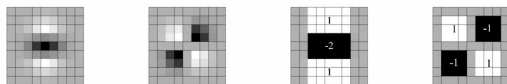
Figure 2: Left: two filters based on Gaussian derivatives. Right: their approximation using box filters.
