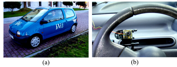
Figure 1: (a) IvvI vehicle, (b) Driver's camera.
