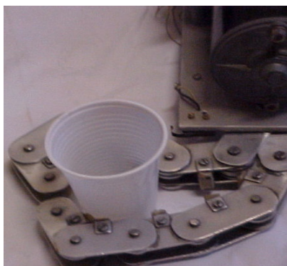
Figure 3: The hyper-redundant gripper of the arm.
