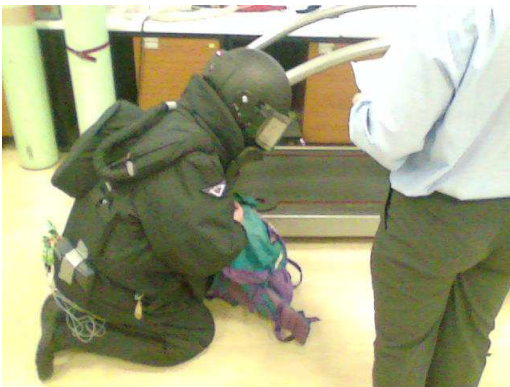
Figure 7: Second activity: kneeling while removing weights from a sack. The wired-in data logger can be seen taped onto the subject's lower back.
