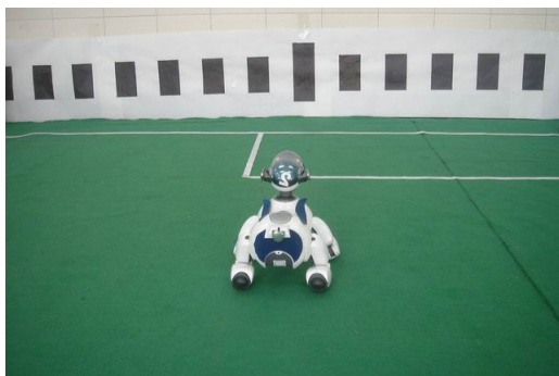
Figure 3: The white board with parallel black bars for body adjusting of the AIBO robots.
