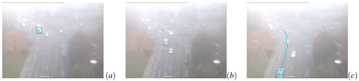
Figure 5: (a): Initial images with their selected object. (b): Results with HSV segments. (c): Results produced with our segments.
