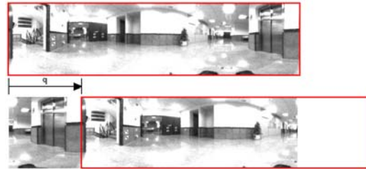
Figure 1: A robot rotation on the ground plane produces a shift in the panoramic image captured.
