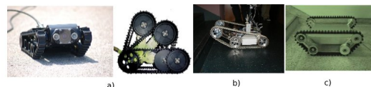
Figure 3: a) Micro VGTV (manufacturer: Inuktun Ltd) b) B2P2 prototype c) VGSTV mechanism.
