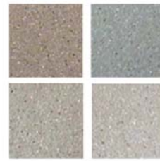
Figure 2: Fragments of high resolution floor images (768x576 pixels) under different light conditions corresponding to 300, 800, 1400 and 2000 lx, respectively.
