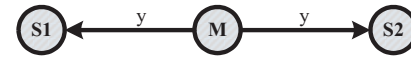
Figure 3: Single master node M and two slave nodes S1 and S2 configuration.
