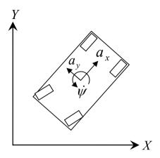
Fig. 2. IMU signals and axes.
