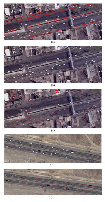
Fig. 8. Vehicle detection and Road Extraction results. (a)(d) The sample image of road segments. (b)The road extraction result, (c)(e)The Vehicle detection result, for image shown in (b), where lines represent extracted roads and for image shown in (c)(e), where dots represent detected vehicles.
