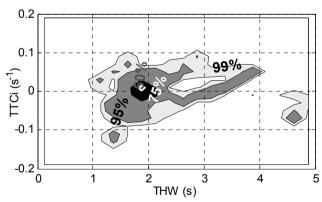
**Fig. 7.** Frequency contour of *THW* and *TTCi* during system control.
