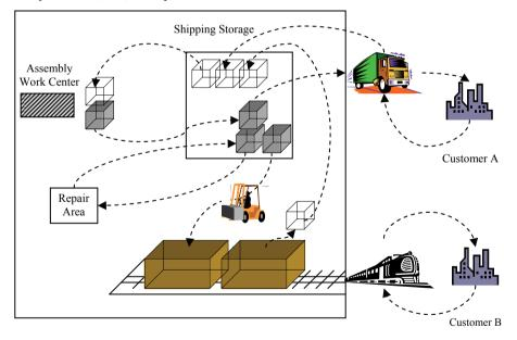
Fig. 1. Schematic of the flow of racks associated with the given work center.
