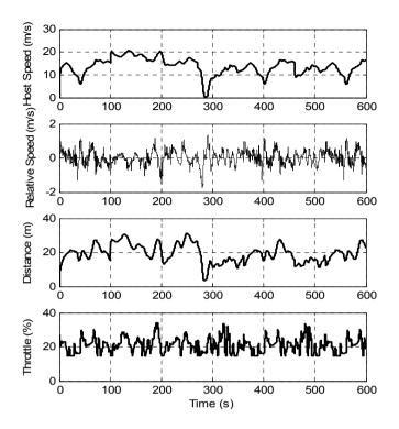
Fig. 4. Data sequences of driver manual car-following.
