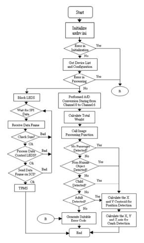
Fig. 3. Interface program flowchart of the integrated system.
