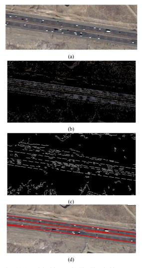
**Fig. 3.** Road Extraction (a) An original image (b) The Threshold pre-processing result (c) The Edge detection pre-processing result (d) The Road Extraction result and direction.
