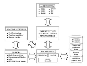
**Fig. 1.** The proposed System Architecture.
