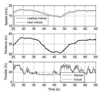
Fig. 6. The performance of the system ACC function.
