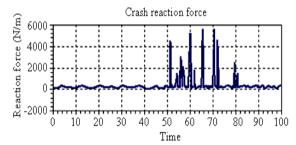
Fig. 5. Vehicle crash reaction forces.
