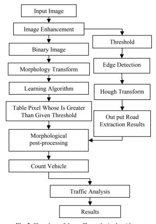
Fig. 2. Flowchart of the traffic analysis algorithm.
