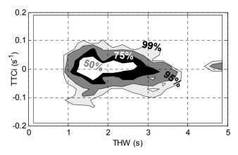
Fig. 1. Frequency contour of THW and TTCi, steady car-following behavior, one driver.
