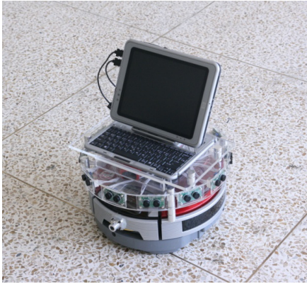
Figure 5: Our overlapped ultrasonic sensor ring prototype.
