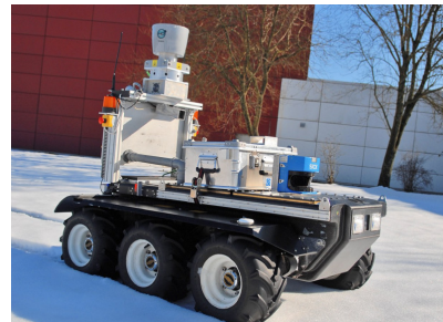
Figure 1: The Quinetiq Longcross robot Suworow equipped with a Velodyne 3D and an additional (unused) 2D laser range finder.
