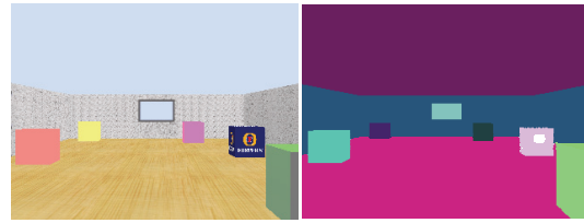
Figure 1: A view of the robot’s random walking sequence. The left image is the original one. The right one shows segments detected during the segmentation phase.
