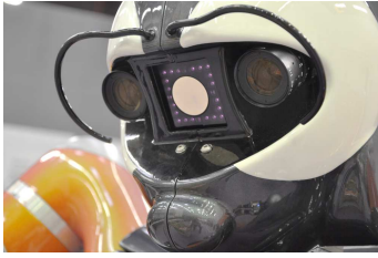
Figure 3: Sensor head: Stereo cameras and 3d-TOF camera mounted on a pan/tilt unit.
