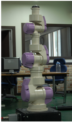
Figure 7: Developed hollow-type robot arm.
