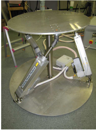
Figure 5: Inclining parallel platform that can rotate around all three axes. The diameter of the platform is 0.7m and is able to carry an adult human.
