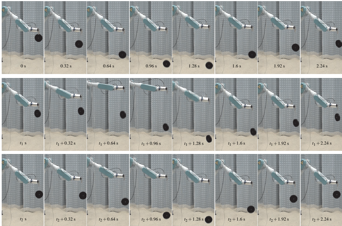
Figure 10: Image sequence of a robotic yoyo. Top sequence present the decent of the yoyo from the gripper. In the middle sequence a behavior of the system after switching from force feedback to vision feedback is shown ( t_1 = 54 s) and in bottom sequence the behavior in steady state is presented ( t_2 = 81 s).
