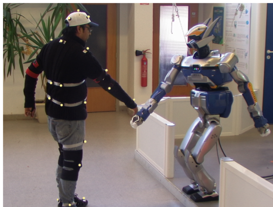
Figure 1: Picture of a human performer extending a handshake and the humanoid robot HRP-2 imitating the gesture. HRP-2 is a 30 Dof, 58 kg, 1.54 m tall humanoid robot manufactured by Kawada Industries, Japan. The human motion was tracked using reflective motion markers and transferred in real-time to the humanoid.
