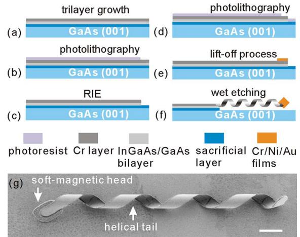
Figure 6: [(a)-(f)] Fabrication procedure of the ABF with InGaAs/GaAs/Cr helical tail. (g) FESEM image of an untethered ABF. The scale bar is 4  $\mu\text{m}$  (Zhang et al., 2009).
