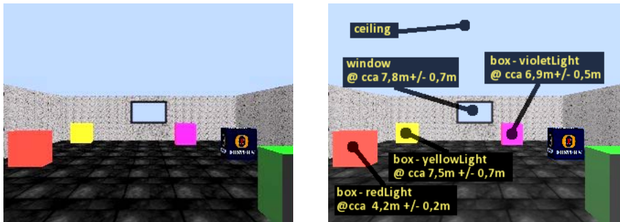
Fig. 4. The same room with different textures (left) and resulted interpreted image (right).
