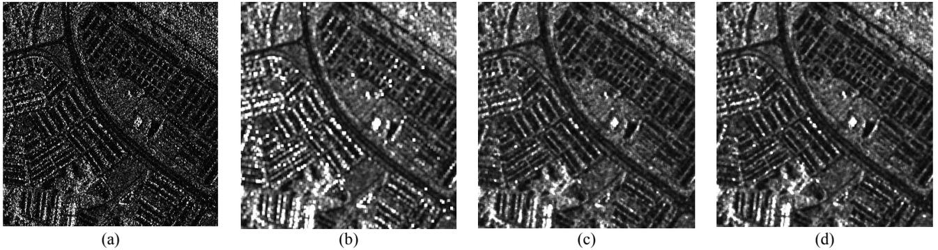
Fig. 1. Filtering results of TerraSAR-X HH intensity over a built-up area, where the filtering was performed using a  $5 \times 5$  window. (a) Unfiltered HH intensity. (b) Boxcar filter, which computes the average dual-polarization matrix as filtering output using all pixels within the test window. (c) Proposed filter ( $\alpha = 0.25$ ). (d) Proposed filter ( $\alpha = 0.05$ ).
