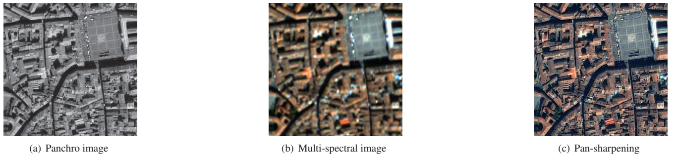
Fig. 2. Pan-sharpening example: high resolution of the panchromatic image are introduced in the multi-spectral image to obtain a multi-spectral high resolution image.
