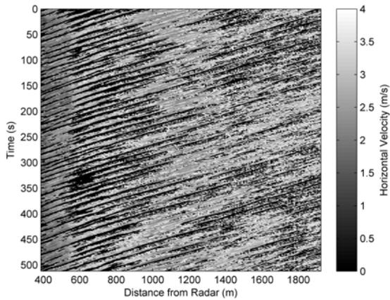
Figure 1. Time – range map of horizontal Doppler speed of a 10min wave observation.
