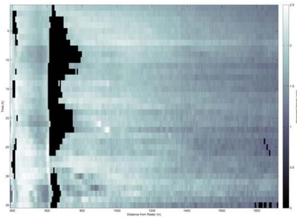
Figure 2. Time - range map of the standard deviation of the horizontal speed covering 40 hours with a 10 minutes average each hour for 40 hourly samples as function of the distance from the radar.
