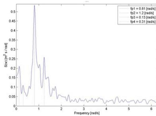
Figure 3a-b. Left: The spectrum of the horizontal velocity measured by buoy. Right: The spectrum of the horizontal velocity measured by radar; the distance from radar is approximately 1200m.
