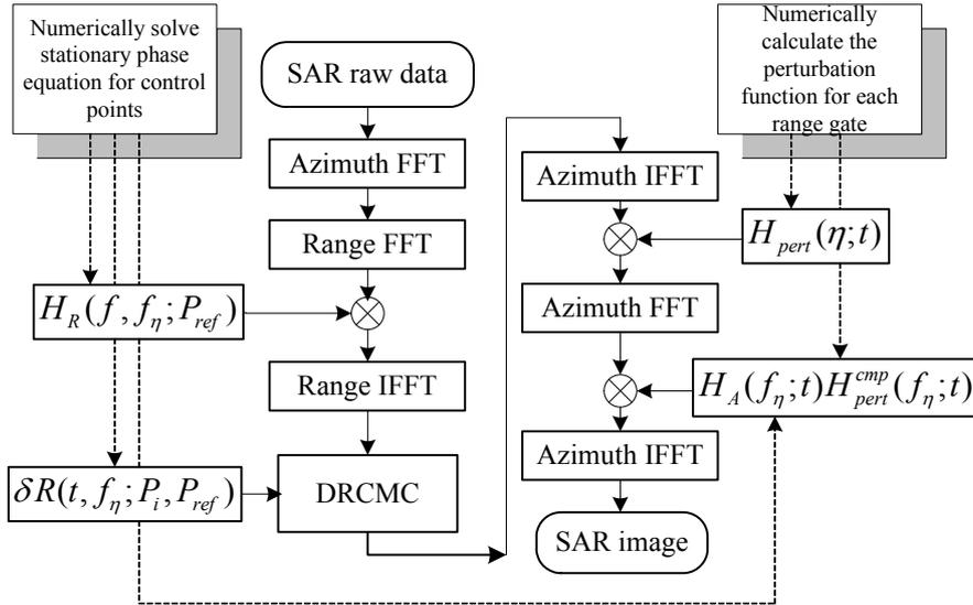
Fig.1 Block Scheme of NuSAR for translational variant bistatic SAR
