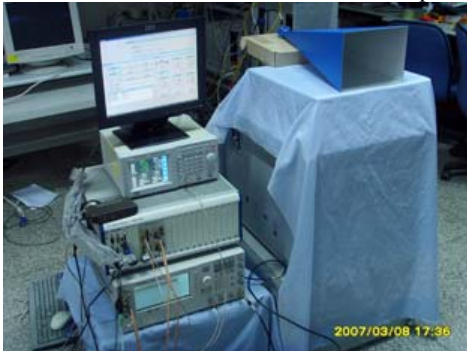
Fig.2 The synchronization unit of the receiver
