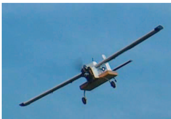
Figure 1. R/C aircraft carrying the ARIEL radiometer during a flight.
