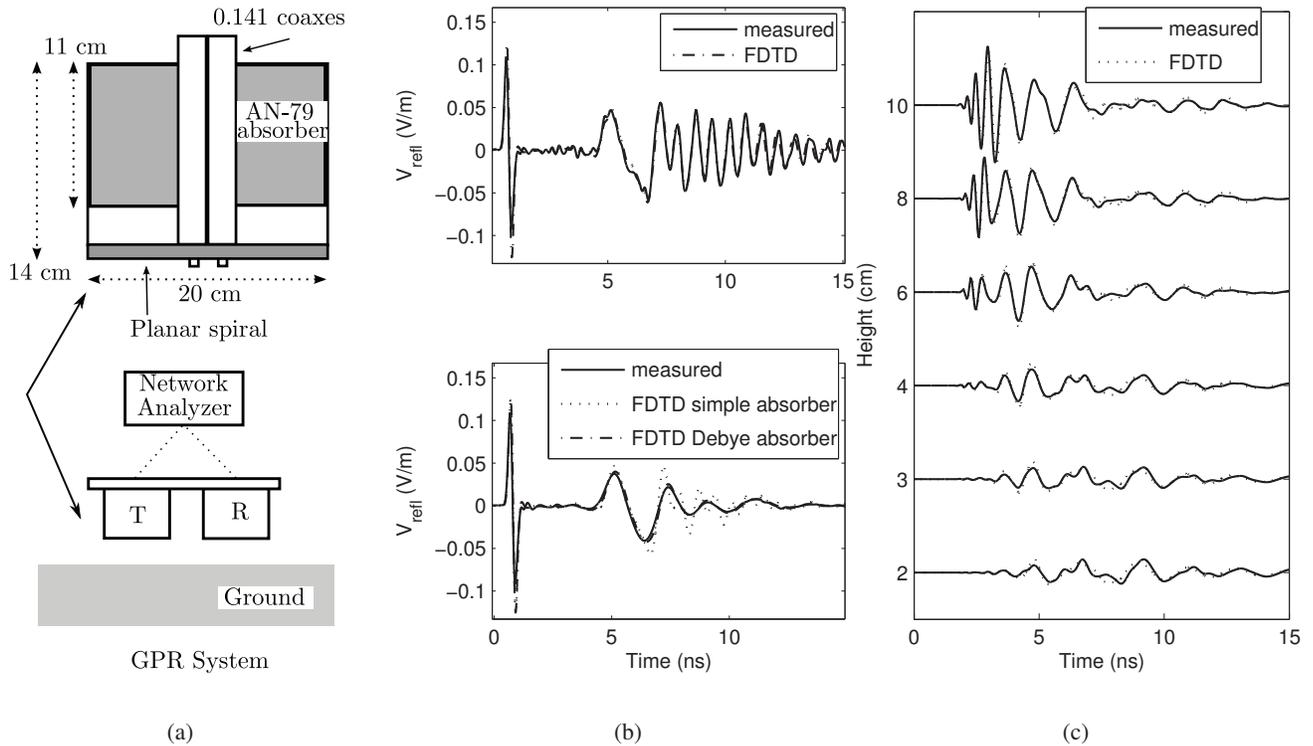
**Fig. 1.** (a) Geometry of the spiral element and the bistatic GPR system. The sizes of the 0.141 semi-rigid coax lines are exaggerated for clarity. (b)  $V_{\text{refl}}$  measured and modeled for the spiral antenna element with an empty can (top) and with the absorber (bottom). The FDTD simple absorber curve is the predicted response using a purely conductive material model. (c) Reflection from the ground on the receive antenna for various heights from the ground, modeled and measured.
