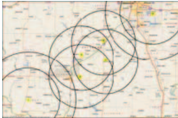
The layout and location of the IP1 weather radar network. The coverage circles of IP1 radar are in radius of 40km. KTLX is to the northeast of the test bed and KFDR is to the southwest of the test bed.
