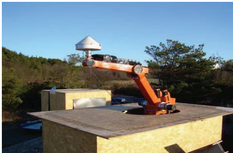
Fig. 1. The installation of a GPS antenna mounted on an industrial robot simulating the displacement of the earthquake.
