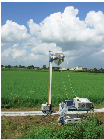
Figure.1 GB-SAR measurement in a paddy field
