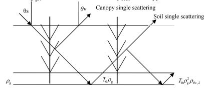
Fig. 1. Interactions of photons with canopy and soil background
