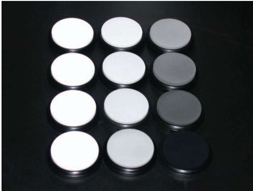
Fig.1: The set of twelve Spectralon samples
