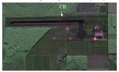
Fig. 2 Pi-SAR2 mode1 RGB power composite image (R:HH, G:HV, B:VV)('08/12/1). Image area is 1.5km x 0.9km
