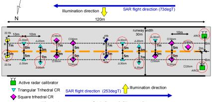
Fig. 1 Arrangement of ARCs and CRs on the runway
