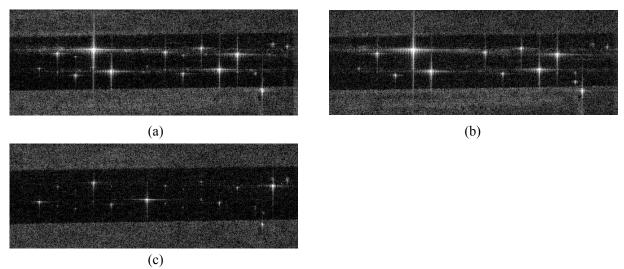
Fig. 3 Pi-SAR2 mode1 image (a: HH, b: VV, c: HV)('08/12/1). Image size is 160m x 60m. Pixel spacing is 0.25m x 0.25m.
