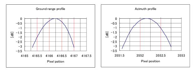
Fig. 4 Up-sampled range profile (left) and azimuth profile (right) of a CR (50cm-square). Pixel spacing is 0.25m x 0.25m.
