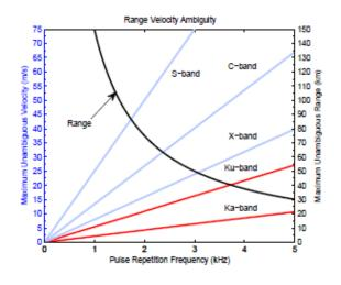
Figure 1: The relation between maximum unambiguous range and maximum unambiguous velocity for different operating frequencies.
