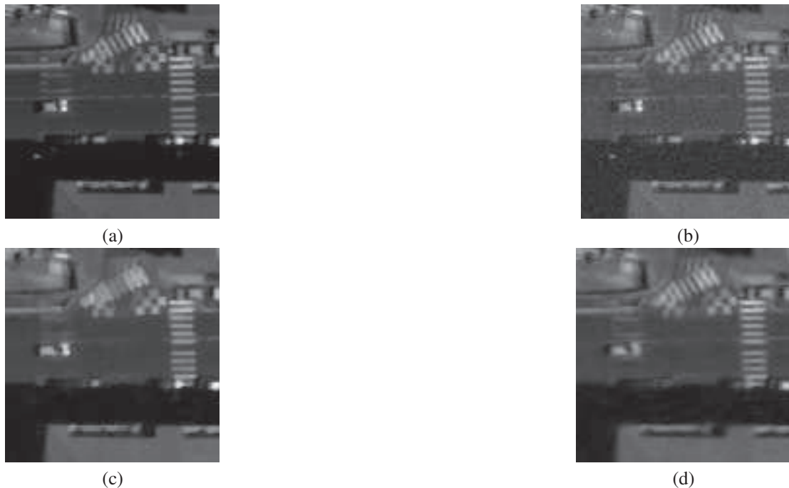
Fig. 1. Restoration of an irregularly sampled, blurred and noisy image. (a) Original image ©CNES, (b) distorted image (Gaussian noise, SNR = 15.62 dB), (c) result with the TV regularization ( SNR = 24.09 dB), and finally (d) result with the DTCW regularization ( SNR = 24.42 dB).
