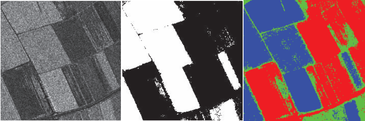
Figure 1: a: Initial image b: Segmented image after Otsu's method c: Segmented image after k-means method
