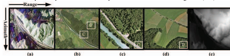
Figure 2 (a) POLSAR image (dB) of Traunstein, 1024×1024 pixel, (Red= |HH-HV| , Green= |HV| , Blue= |HH+VV| ) (b) Optical image of Traunstein (Google Earth) (c)-(d) Heavily forested areas: Data C, Data D (e) DEM image
