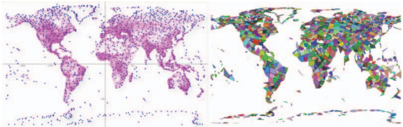
Figure 3. Clustering results. 1265 clusters in 125 ms with threshold, \delta of 0.05. (Left) shows actual points in purple and cluster points as dark blue dots. (Right) shows polygon extents of each cluster point.
