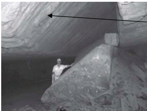
Figure 3. A block that fell out of the hangingwall along a flexural slip fault (Perrit and Roberts [3]).
