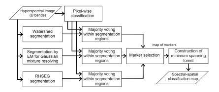
**Fig. 1**. Flow-chart of the proposed *MSSC-MSF* classification scheme.
