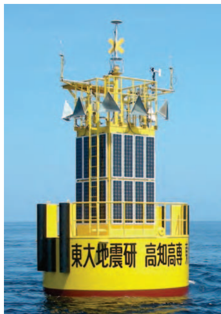
Figure 2: GPS buoy installed offshore of Cape Muroto, Japan
