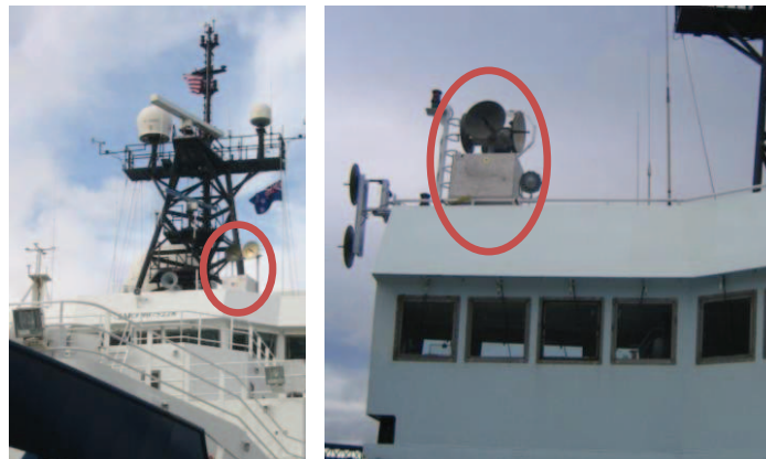
Figure 1. Coherent, X-band radars mounted on the R/V Revelle (left) and the R/V Thompson (right).
