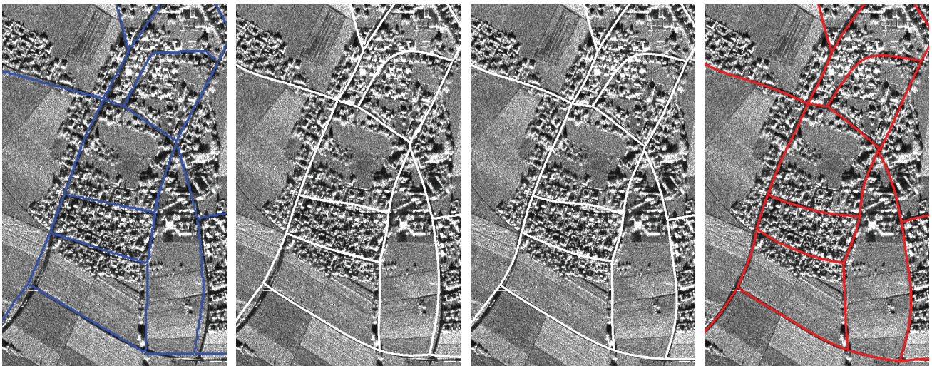
Figure 2: Geometric refinement of a road network from an airborne SAR image using network snakes: initialization (blue), optimization steps (white) and final result (red)
