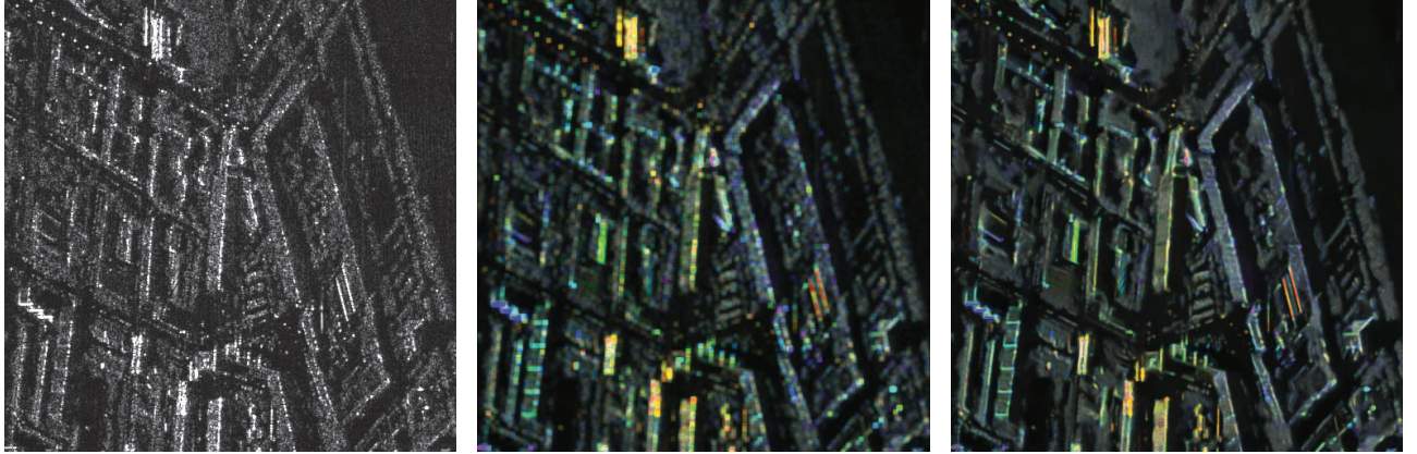
Fig. 1. PolSAR images of Dresden (Germany) sensed by E-SAR ©DLR obtained from (a) the single-look complex HH SAR image, (b) the boxcar estimator and (c) the NL-PoSAR filter. The colorization is based on intensity and entropy-alpha decomposition.
