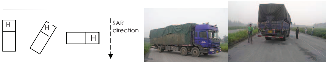
Figure 2: The distribution diagram of vehicles 180^\circ, 225^\circ, 270^\circ (from left to right) in Experiment 2
