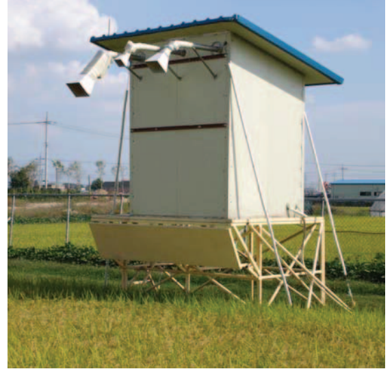
Fig. 1. View of L, C, X-band automatic scatterometer system.
