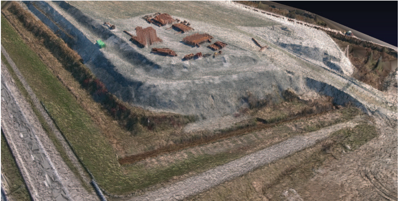
Fig. 5. Close-up of the dense generated 3D model, showing part of the highway and the complex shape of the hill. This subsection contains around 1 million vertices.
