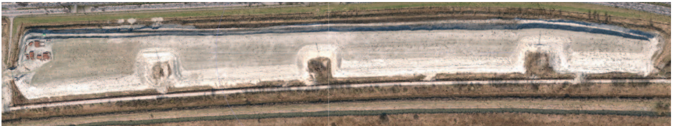
Fig. 4. Orthophoto created by viewing the generated 3D model top-down, measuring approximately 1000m x 200m.
