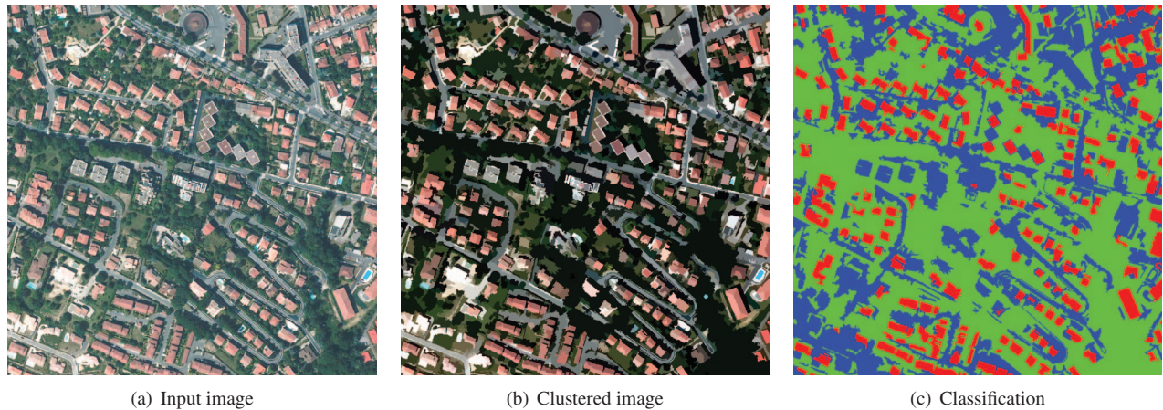
Fig. 2. Results obtained after a few iterations on a pan-sharpened Quickbird patch with less than 10 examples per class
