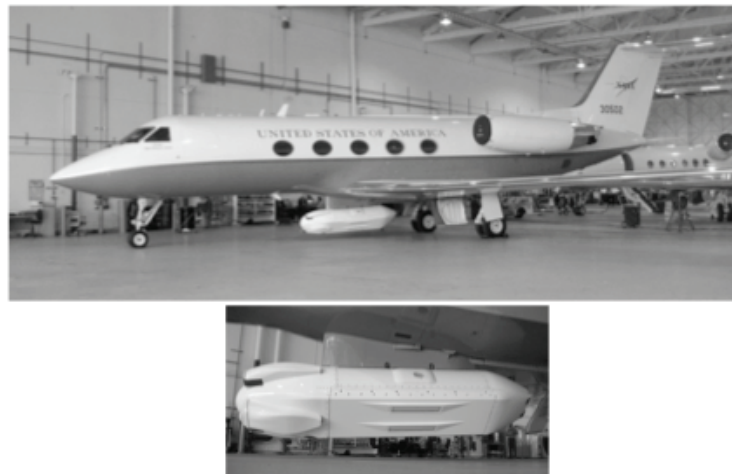
Figure 1: Picture of NASA Gulfstream III with pod configured for Ka-band interferometry. Lower insert shows close-up with details of the two antennas.
